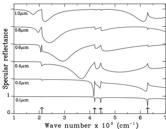
FIG. 2. Calculated specular reflectance of a gold grating with the parameters as defined in Fig. 1. This magnitude is analyzed as a function of the wave number of the incident light for increasing values of the depth of the grooves going from  $h = 0.1\text{--}1.0 \mu\text{m}$ . For the sake of clarity each curve is shifted by +1 with respect to the previous one.
