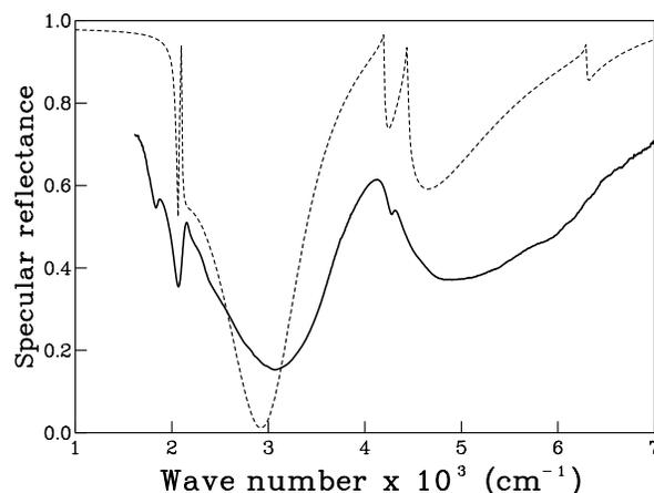
FIG. 4. Experimental (full line) and computed values (dashed line) of the specular reflectance of a gold grating with grooves of depth  $h = 0.6 \mu\text{m}$ , period  $d = 3.5 \mu\text{m}$ , and width  $a = 0.5 \mu\text{m}$ . The angle of incidence is  $21^\circ$ .
