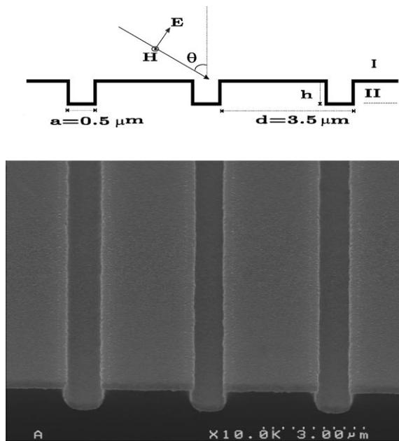
FIG. 1. A scanning electron micrograph of a sample that consists of a metallic grating with grooves of depth  $h = 0.2 \mu\text{m}$ . In the upper part of this figure we show a schematic view of our samples with grooves of width  $a = 0.5 \mu\text{m}$  and separated by  $d = 3.5 \mu\text{m}$ . The incident light is  $p$  polarized and the angle of incidence  $\theta = 21^\circ$ .
