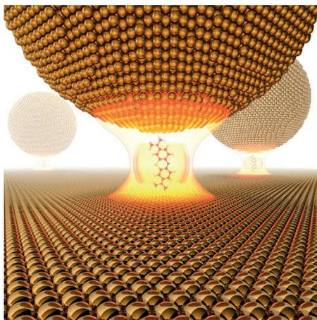
**Figure 2** | Illustration of a particle-on-mirror plasmonic cavity strongly coupled to a single molecule placed within its (sub-)nanometric gap. Figure reproduced from ref. 20, Nature Publishing Group.
