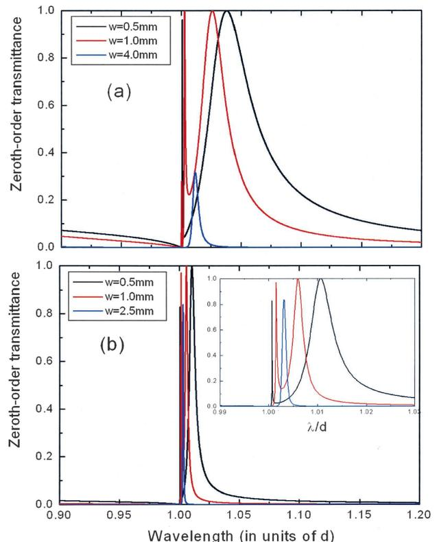
Fig. 2. Theoretical zeroth-order transmittance spectra corresponding to different infinite hole arrays with (a)  $R = 1.25$  mm and (b)  $R = 1$  mm. The inset in (b) represents the same physical quantity but for a smaller range of wavelengths.
