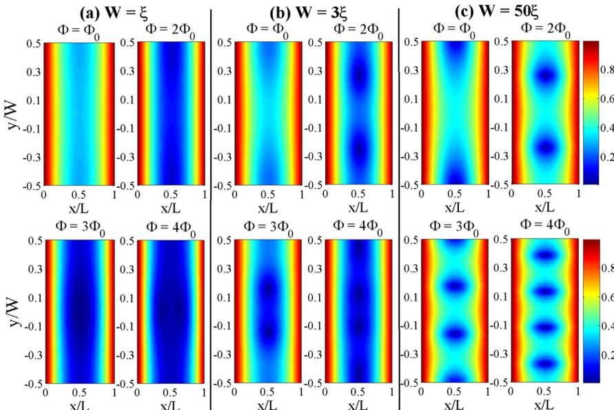
FIG. 2 (color online). Spatial map of the modulus of the pair correlations,  $|F(\mathbf{R})|$ , for  $L = 2\xi$  and  $\phi = 0$ . The different panels correspond to different values of the width  $W$  and the magnetic flux  $\Phi$ , as indicated in the graphs.  $|F(\mathbf{R})|$  has been normalized to its value inside the electrodes, the temperature is  $k_B T = 0.01\Delta$ , and perfect transparency was assumed.
