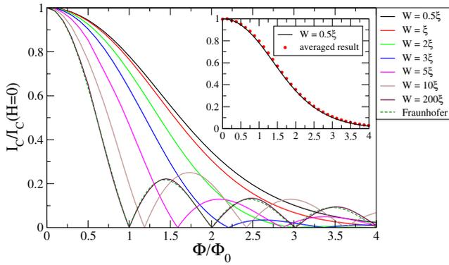
FIG. 3 (color online). Critical current normalized by the zero-field value vs magnetic flux for a wire length  $L = 8\xi$ , perfect transparent interfaces,  $k_B T = 0.01\Delta$ , and different values of  $W$ . The dashed line shows the standard Fraunhofer pattern given by  $\sin(\pi\Phi/\Phi_0)/(\pi\Phi/\Phi_0)$ . The inset shows for  $W = 0.5\xi$  the comparison between the exact result and the approximation used for the narrow-junction limit.
