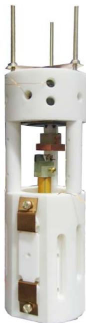
Fig 1. Photograph of the AFM detached from the dilution unit showing the scanning piezotube assembly and sample holder.
