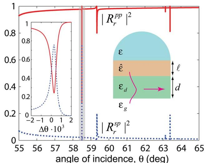
Fig. 4. (Color online) Reflection coefficients for hybrid-mode spectroscopy in a waveguide in K geometry with  $\ell=0.7\lambda$ ,  $d=\lambda$ ,  $\epsilon_d=5.5$ , and  $\epsilon_g, \epsilon, \hat{\epsilon}$  as in Fig. 1. The inset represents the zoom of the highlighted region with  $\Delta\theta=\theta-\theta_0$  and  $\theta_0=58.497^\circ$ .
