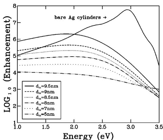
FIG. 4. The local enhancement of the Raman signal evaluated at the region between the nanotubes, for different values of  $d_{in}$  and as a function of the energy of the incoming photon. The same quantity, as evaluated for bare Ag cylinders of diameter 9.5 nm and separated by 10.3 nm, is also shown.
