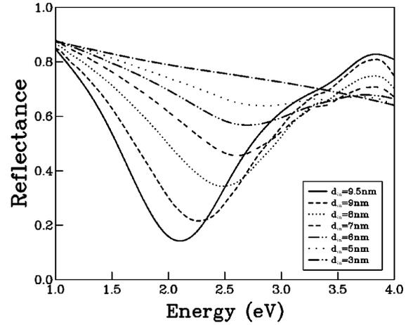
FIG. 2. Calculated optical reflectance of the structure shown in Fig. 1 for a normally incident photon of frequency ranging from 1 to 4 eV, and different values of the inner core filled with silver,  $d_{in}$ .
