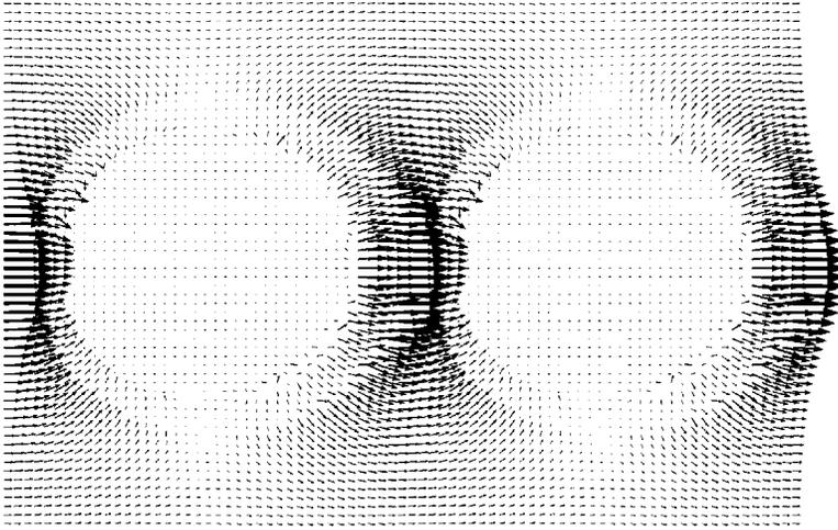
FIG. 3. A detailed picture of the total  $\mathbf{E}$  field generated by a normally incident plane wave impinging on the array of Ag-filled carbon nanotubes of Fig. 1 with  $d_{\text{in}}=8$  nm. The  $\mathbf{E}$  field is evaluated at  $\omega=2.5$  eV, the frequency at which the optical reflectance is minimum for this case. The total  $\mathbf{E}$  field is shown for two unit cells of the array.
