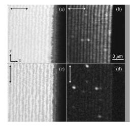
FIG. 9. FH (a),(c) and TPL (b),(d) images of a gold particle array on glass with  $\Lambda_x$ =860 nm,  $\Lambda_y$ =430 nm, and  $d_x=d_y$ =160 nm obtained using 3 mW of incident power at the wavelength of 760 nm for the polarizations indicated by arrows on the images. The maximum TPL signal is (b) ~6200 and (d) ~2000 counts/s.
