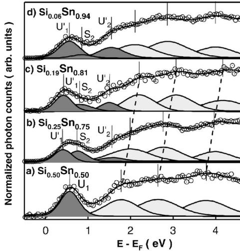
FIG. 11. KRIPES spectra obtained at normal incidence for (a) the  $\gamma$  phase, (b) the intermediate phase close to the mosaic phase (interm1), (c) an intermediate phase close to the  $\alpha$  phase, and (d) the  $\alpha$  phase.
