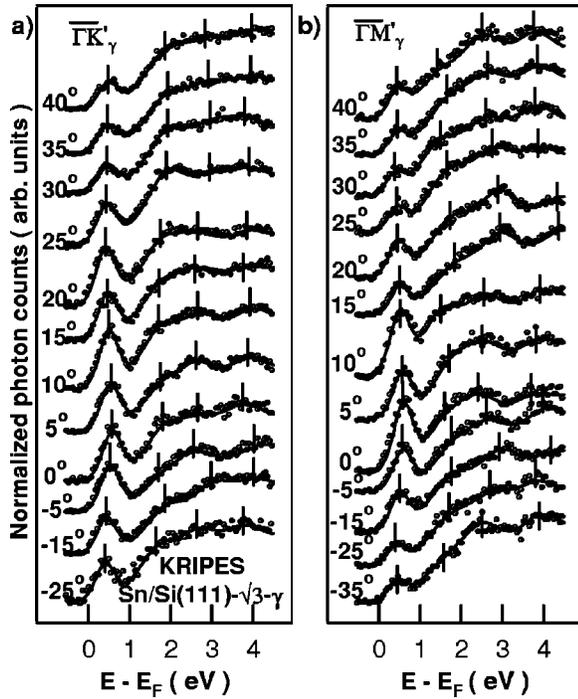
FIG. 8. KRIPES spectra of the  $\gamma\text{-}\sqrt{3}$  (mosaic) reconstruction along the directions  $\overline{\Gamma K'}$  (a) and  $\overline{\Gamma M'}$  (b) of the SBZ for selected positive and negative angles of the incident electrons. The vertical bars represent the position of the maximum of each Gaussian.
