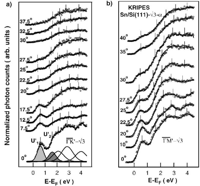
FIG. 3. KRPES spectra of the  $\alpha$ - $\sqrt{3}$  surface along the  $\overline{\Gamma K'}$  (a) and  $\overline{\Gamma M'}$  (b) directions of the SBZ for selected angles of the incident electrons. Experimental curves are plotted as circles, the fit is represented by a continuous line, and each Gaussian maximum is marked by a vertical bar.
