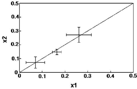
FIG. 12. Si concentration calculated from Figs. 11(b)–11(d) spectra with two different methods:  $x_1$ , first method and  $x_2$ , second method. See text for a description (Sec. IV) of the methods. The concentration  $x_2$  has been obtained with a relative weight of 2/3 for the electronic densities of  $U'_1$  (Sn derived) with respect to  $S_2$  (Si derived).
