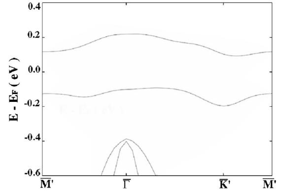
FIG. 2. Surface band structure along the symmetry directions  $M'-\Gamma-K'-M'$  of the SBZ for  $\text{Sn}/\text{Si}(111)-(2\sqrt{3} \times \sqrt{3})$  with one Sn adatom and one Si adatom, simulating the mosaic structure. The lower (occupied) surface band is associated with the Sn dangling bond while the upper (empty) surface band is related to the Si dangling bond. The energy of these bands is indicated with respect to the Fermi level. The surface is semiconducting.
