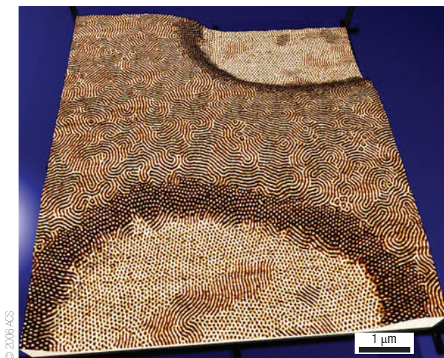
Figure 4 Complex microdomain structure of a block copolymer. The AFM images are rendered into three-dimensions using the height image as height-field and the phase image as contrast. The images show the formation of terraces in a thin film of SBS block copolymer and the systematic change of microdomain structures along the changes in film thickness from 32 nm at the lowest terrace to 57 nm at the higher terrace. Reprinted with permission from ref. 54.
